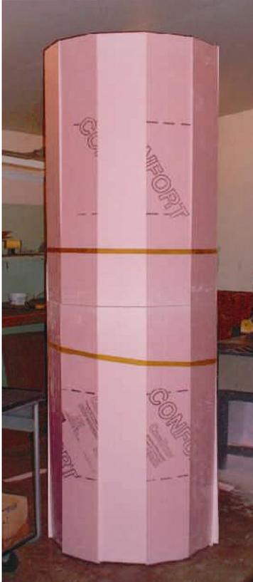
This shows the two 4' sleeves together, making it 8 feet long. The yellow straps are what we use to hold the sleeves while the glue dries.
