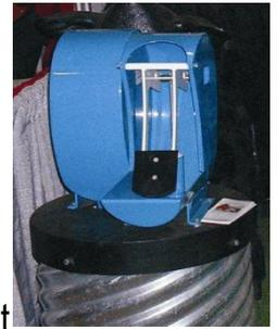
1. Cut a 25½" diameter circle (for a 24" culvert) from a sheet of 10 gauge metal. It is safest to verify the outside dimension (OD) of your culvert because they will vary. Make the circle slightly larger than the OD measurement (including the depth of the ribs). A larger culvert will require heavier gauge steel, to reduce flexing. **Always build the lid with the crown up so water flows off.**
