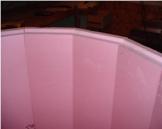
Note how the edges on this sleeve are the opposite of the edges on the sleeve above – making a match when you put one over the other.
