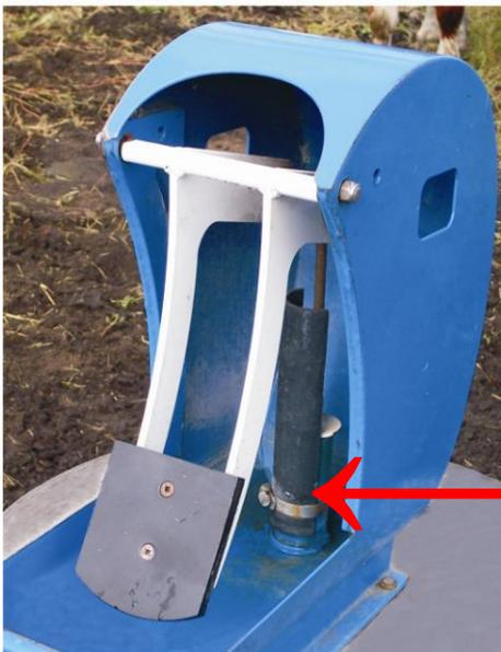
The water diverter will direct the water flow to the back only.
